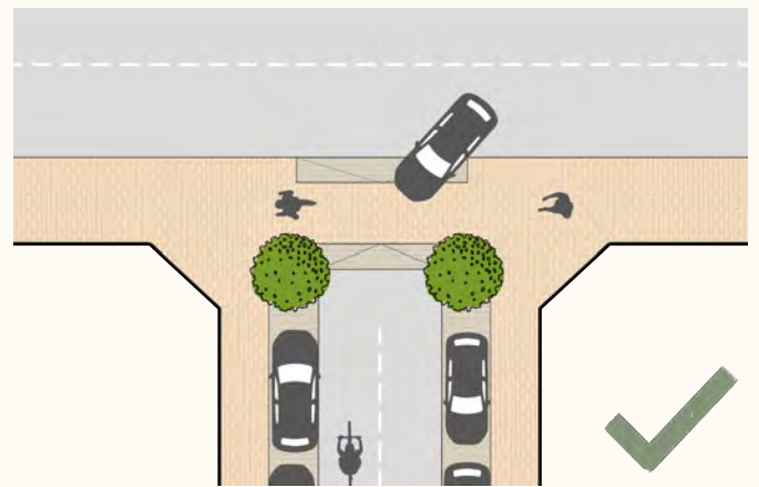
A conventional side street junction (top) compared to a continuous, or Copenhagen, crossing (bottom).
