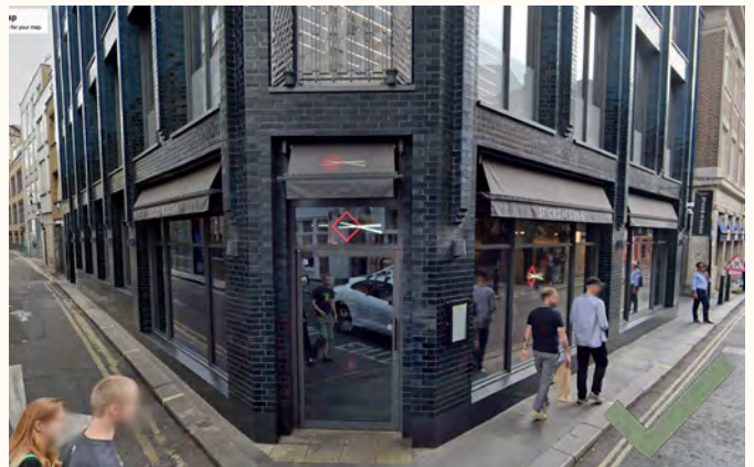
Contemporary retail and shopfronts must still use brick or stone to define the openings.
